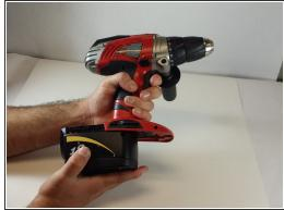
While holding down the red locking switch, slide the battery towards the back of the drill until the battery is fully removed from the drill.
