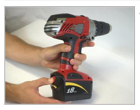
Grip the drill. Locate the red locking switch on the back of the battery.
