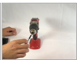
The chuck sleeve is held on by a 20mm Phillips #2 screw in the center. This screw is reverse threaded. Insert a Phillips #2 screwdriver and rotate it clockwise to loosen and remove it.
