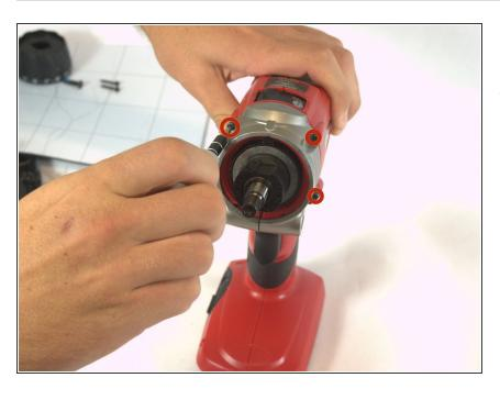
Remove the 4 20mm T10 Torx screws. Insert a T10 Torx screwdriver and turn counterclockwise.
