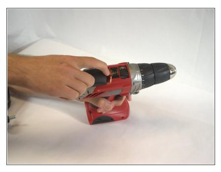
Hold drill upright with one hand and slide the gauge backwards to remove it with the other.
