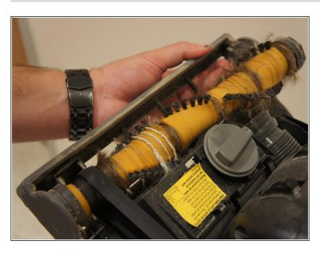
Firmly press upwards from below the brush roll on the side opposite the belt.
