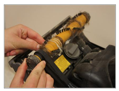
After one end is displaced, remove the other side by pressing firmly upwards from below the the brush roll.
