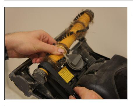
Once the brush roll is displaced from the base, detach the belt from the brush roll in order to clean the brush roll.
