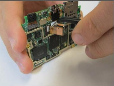
Remove camera from back of the motherboard with tweezers.
