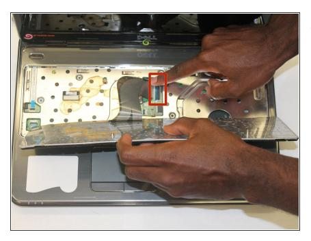
Pull the black tab up and then pull left on keyboard plug to release keyboard.
