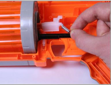
In order to remove the white plastic holder, you must remove the spring that keeps it in place.
