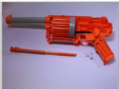
Using your hand, slide the track out of the gun by pulling it away form the device.
