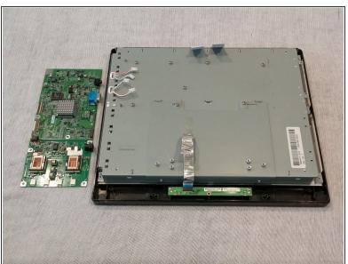
Lift and remove the joined Power Supply and Video Display boards.
