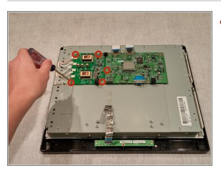
Unscrew the 5 screws holding the joined Power Supply and Video Display boards on.
