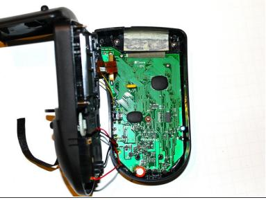
Gently pull the access panel up to separate from the device
