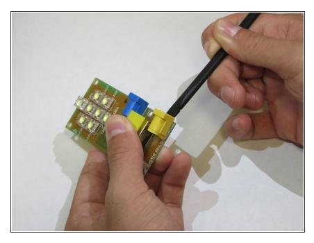
• Use the flat end of the spudger to pry the charging terminal away from the motherboard.
