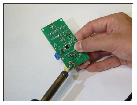
Start melting the solder on each prong connector individually with the soldering iron.
