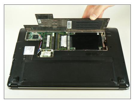
Gently lift the back panel from the side closest to the battery and remove panel
