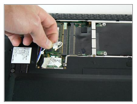
Remove white and black wires to make room to remove the second RAM module.
