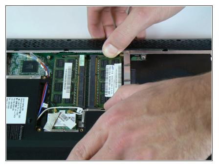
• Push retention clips outward and then gently slide out of slot
