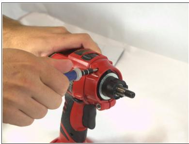
Locate 4 screws on side of the drill. Remove using Torx T10
