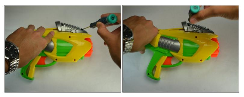
• Using a screwdriver, remove the two 11.6 mm phillips 00 screws holding the grey slider together.
