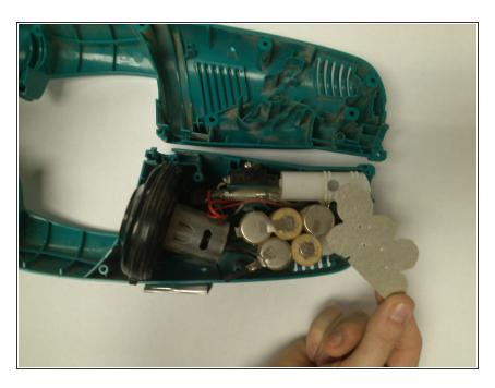
Remove the silver-colored battery cap from the top of the battery.
