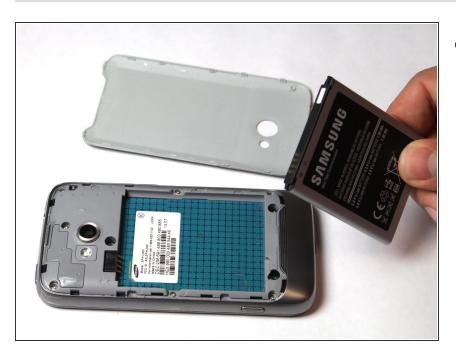
Remove battery from slot.
