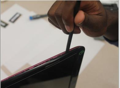
Use a spudger to separate and remove the plastic frame on the front of the screen.
