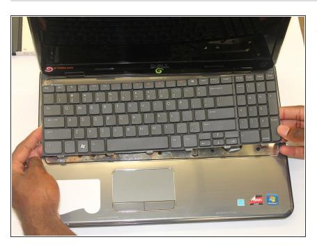
Lift the keyboard up slightly and push forward in order to release bottom tabs.
