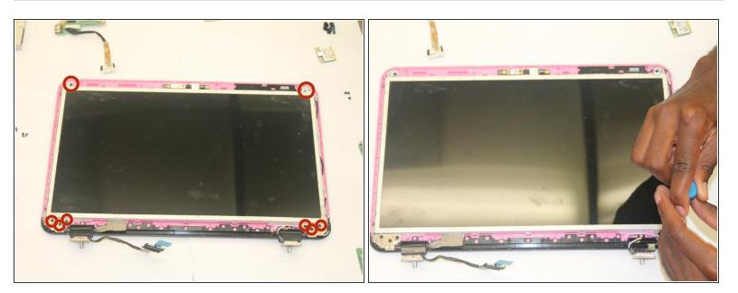
Use a Phillips #000 Screwdriver to remove the 8 6.0mm Phillips #000 screws marked in the image.
