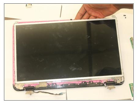
Lift LCD screen from the plastic frame.
