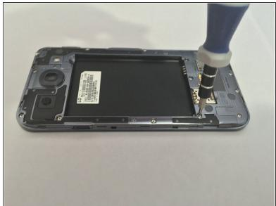
• Make sure you remove the battery first. You will see that there are 14 screws on the back of the inner case. Use the Phillips head screwdriver to remove each of the screws, make sure to put the screws in a safe place where they will not get lost.
