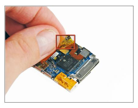
Peel back the orange tape covering the camera ribbon cable up off the logic board.
