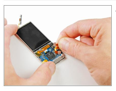
Lift and remove the camera from the logic board.
