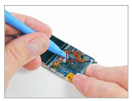
Use an iPod opening tool to pry the camera connector off its socket on the logic board.
