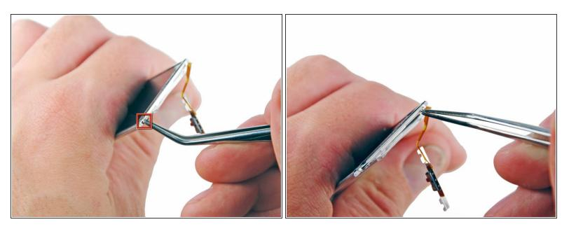
Use a pair of tweezers to bend back the metal clips at the top of the display.
