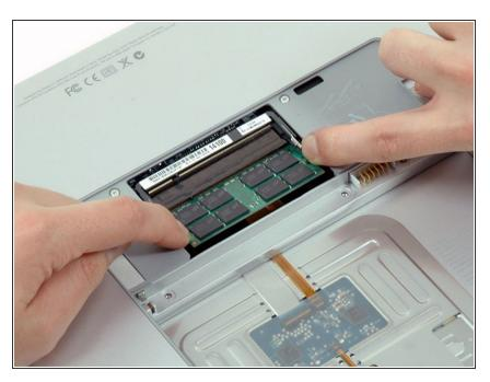
Release the tabs on each side of the RAM chip at the same time. These tabs lock the chip in place and releasing them will cause the chip to "pop" up.
