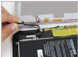
Remove the speaker cable from its socket by gripping both sides of the white connector piece with tweezers and pulling straight out.
