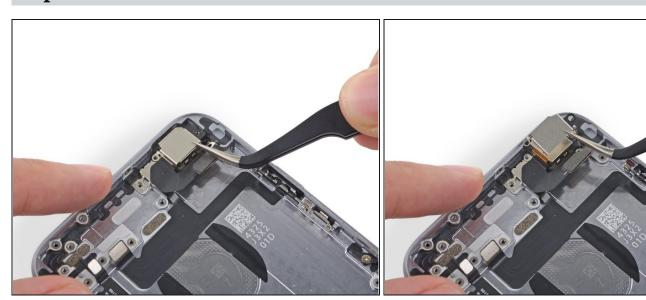
• Remove the rear-facing camera bracket.
