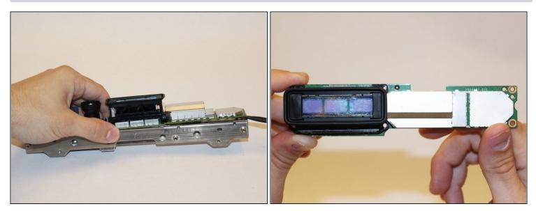
• Using the spudger, detach the IR blaster board from the heatsink.
