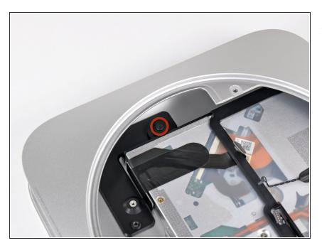
Remove the 7.9 mm T6 Torx screw securing the optical drive to the outer case.
