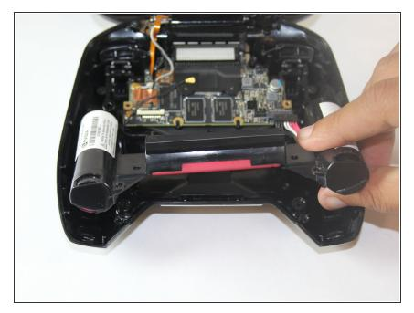
Pull the battery apparatus out once all cables are removed.
