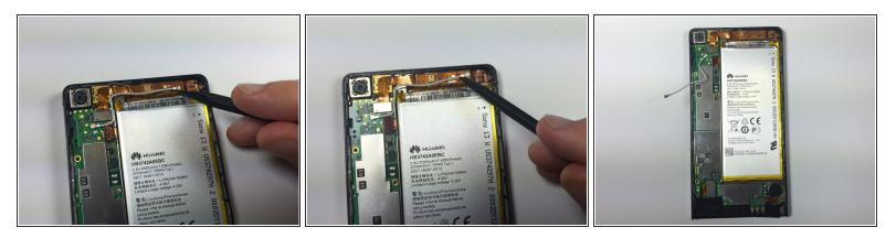
• Use the pointy end of a spudger to pry the antenna connector off of its socket.
