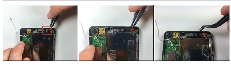
Use tweezers to lift the rubber alignment tab out of its frame.
