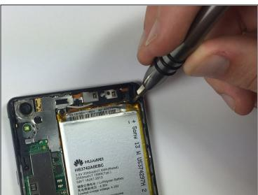
• Push down the yellow plastic lining at the top of the battery and remove the two 2.5mm Phillips #000 screws.
