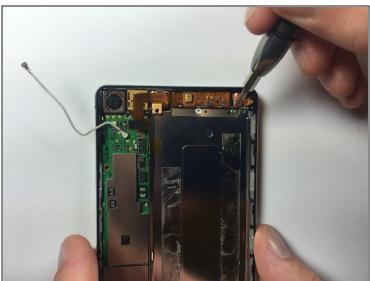
Remove the two 2mm Phillips #000 screws securing the copper flex cable to the silver metal tab.
