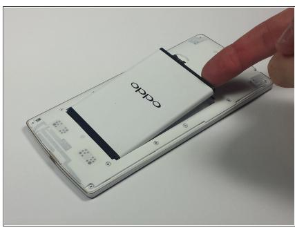
With your finger, remove the battery from the phone by gently lifting the top-right corner nearest to the camera. To reassemble your device, follow these instructions in reverse order.
