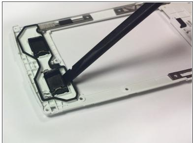
Using the flat end of the spudger, pry the speaker drivers off of the chassis.
