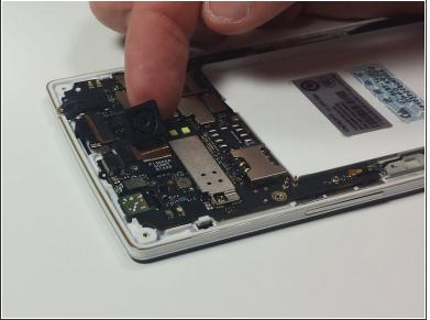
• Use your fingers to pull the camera straight up from the motherboard to fully detach the camera.
