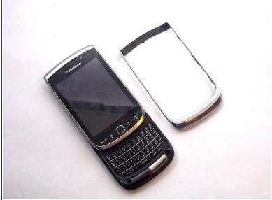
Remove front silver trim by using plastic opening tools and wiggle it off.
