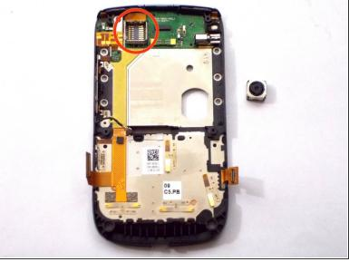
• Use the Phillip screw driver to wiggle the camera sensor out.
