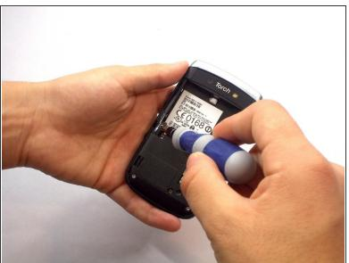
Unscrew the four screws using the T6 screw driver
