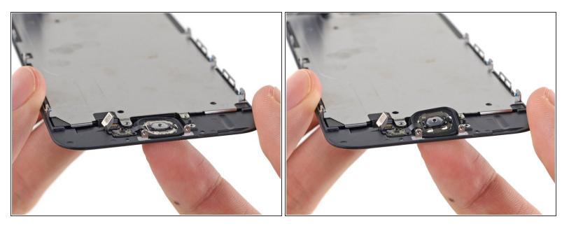
$\bigwedge$  The rubber membrane surrounding the home button is very thin and tears easily.
