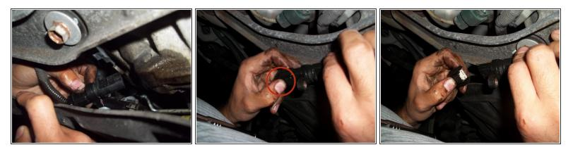
(i) Note the correct position of the sensor so you will be able to insert the new sensor later on.
