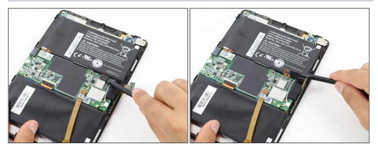
• With the spudger, remove the <u>flat-top connector</u> coming from underneath the motherboard.
