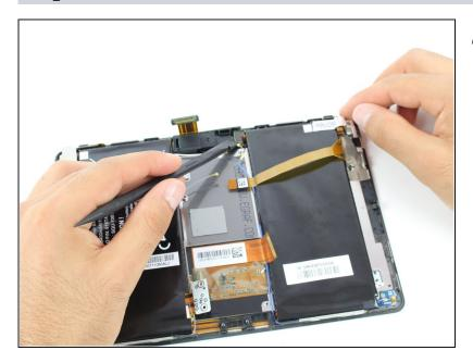
• Use a spudger to detach the <u>flat-top connector</u> from the camera assembly.
