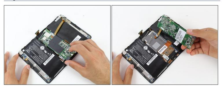
• Gently lift the motherboard away from the device. If there is any resistance, check the previous steps to ensure that all connections have been removed.
