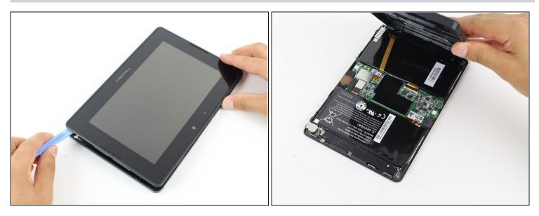
• Use a plastic opening tool to pry the back panel off by inserting it in between the front and back panel.
