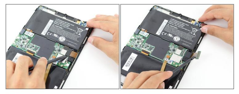
• Remove the <u>flat-top connector</u> coming from across the camera assembly with a spudger.
