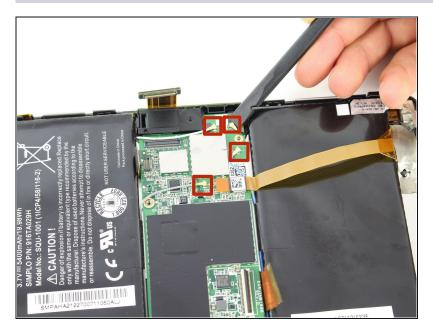
Lift all four <u>antenna</u> <u>connectors</u> from the motherboard again using the spudger.
