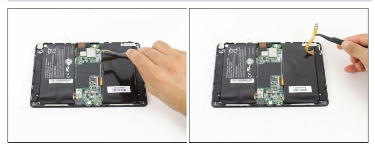
• Remove the battery connector using either your fingers or a pair of <u>tweezers</u>.
