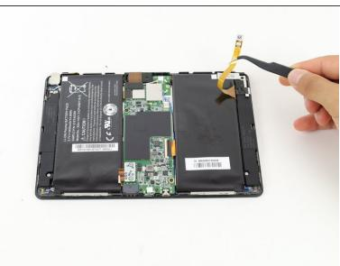
Remove the battery connector using either your fingers or a pair of tweezers.
