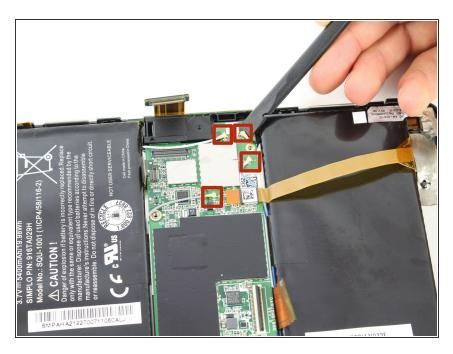
Lift all four <u>antenna connectors</u> from the motherboard again using the spudger.
