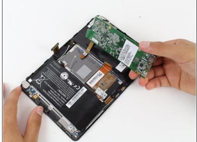
Gently lift the motherboard away from the device. If there is any resistance, check the previous steps to ensure that all connections have been removed.
