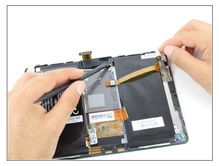
Use a spudger to detach the <u>flat-top</u> <u>connector</u> from the camera assembly.
