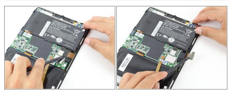
Remove the <u>flat-top connector</u> coming from across the camera assembly with a spudger.
