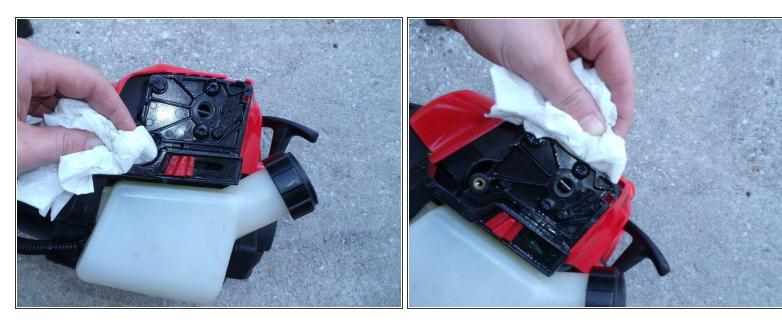
Wipe all oil and water residue around the air filter casing with a paper towel or rag.
