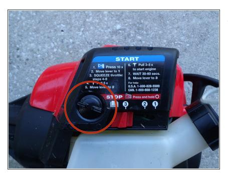
Remove the air filter housing by turning the plastic screw counterclockwise with your hand.
