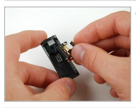
Remove the headphone jack and shuffle switch from the front case.
