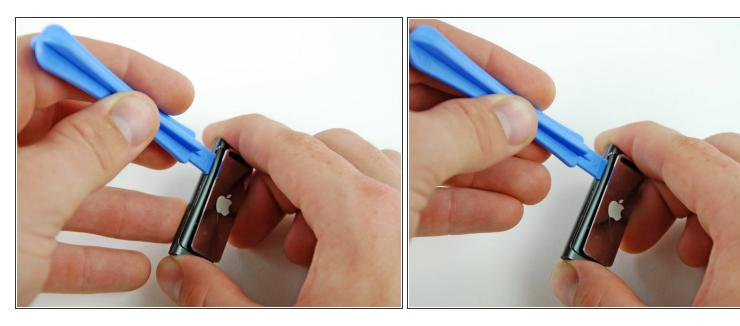
Insert an iPod opening tool into the newly widened gap, and pry the rear case up and away from the front case.
