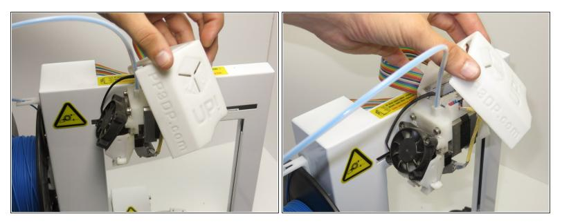
• Remove the 3D printed plastic cover by lifting up and to the left. The latches in the back should lift right out, however this can be tricky since the 3D printed connections don't always sit in place well.
