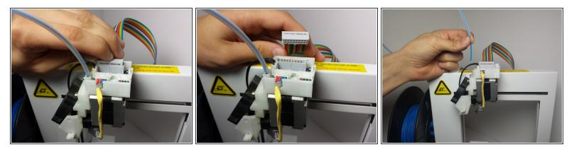
• Disconnect the large colored ribbon cable on the top of the printer by wiggling slightly side to side and pulling up to disconnect.
