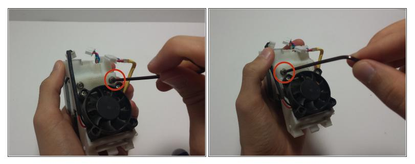
With the 2.5mm hex tool unscrew the two small hex screws immediately above the top left and right corners of the fan.
