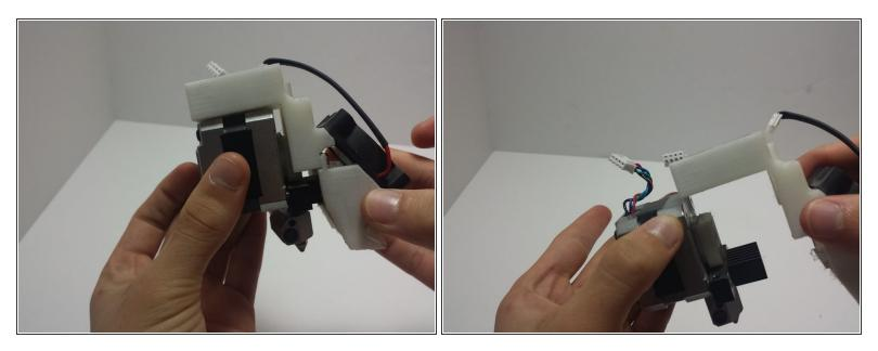
• Once the two screws have been removed the entire plastic body, with fan and connector board, should be able to slide off of the stepper motor by pulling the plastic assembly towards you.
