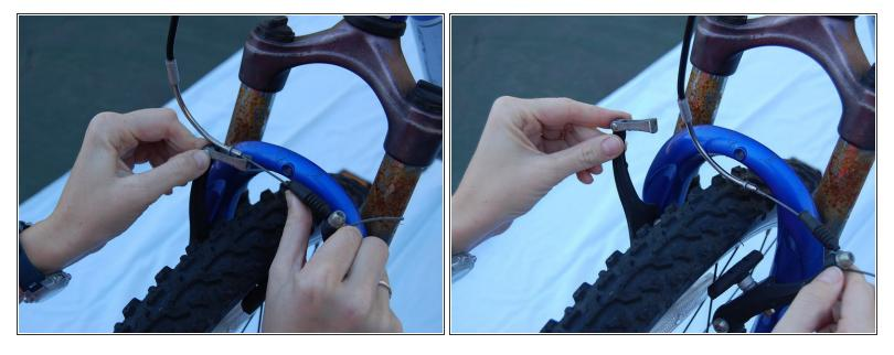
Unhook the brake wire in the metal tube from the brake wire holder on the brake caliper in your left hand.
