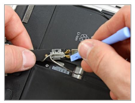
Pry the Wi-Fi and Bluetooth antennas up off their respective sockets on the Wi-Fi/Bluetooth board.
