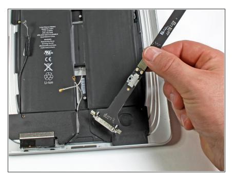
• Remove the dock connector cable from the rear panel assembly.
