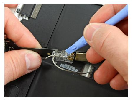
Carefully remove the plastic cover over the WiFi/Bluetooth board and dock connector cable using an iPod opening tool.
