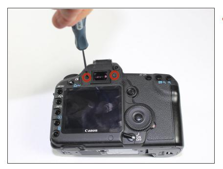
Remove each 6.3 mm screw on either side of the viewfinder using a Phillips #0 screwdriver.
