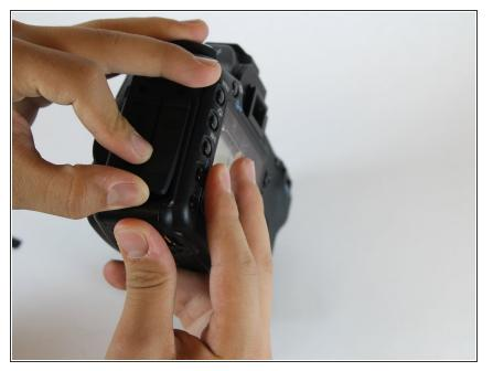
• Lift the rubber flap covering the input/output jacks.
