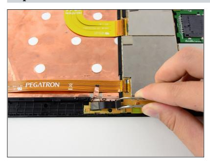
Carefully remove the ribbon cable from the housing by pulling gently upwards on the sides of the cable housing. The cable should come straight up off of its housing.
