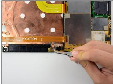
Using tweezers, pull the copper foil up from the back of the camera. It should peel up easily.
