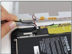
• Remove the speaker cable from its socket by gripping both sides of the white connector piece with <u>tweezers</u> and pulling straight out.
