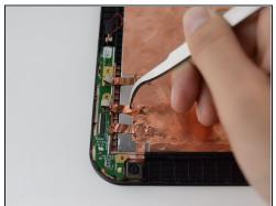
Pull copper tape away from the back, keeping it connected to the green rear camera board.
