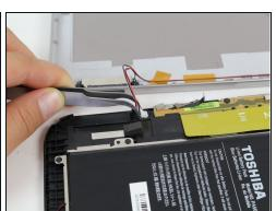
• Remove the speaker cable from its socket by gripping both sides of the white connector piece with <u>tweezers</u> and pulling straight out.
