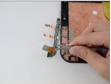
Gently pinch the ribbon cable connector between two fingers or with tweezers and pull
