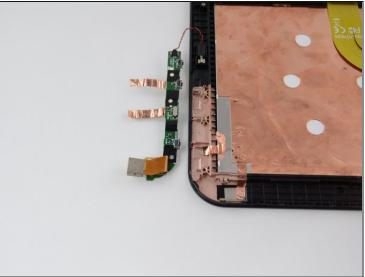
• Using your hands remove daughter board by lifting it off of the tablet chassis. Flip it over and place it next to the tablet face-down.
