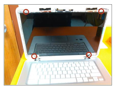
Remove the four screws securing the display panel.
