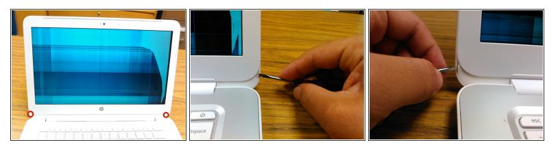
Pry up the nylon covers at the lower left and right of the display to reveal two Phillips head screws.
