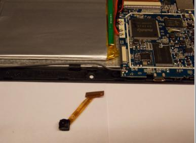
Carefully remove the camera from its housing.
