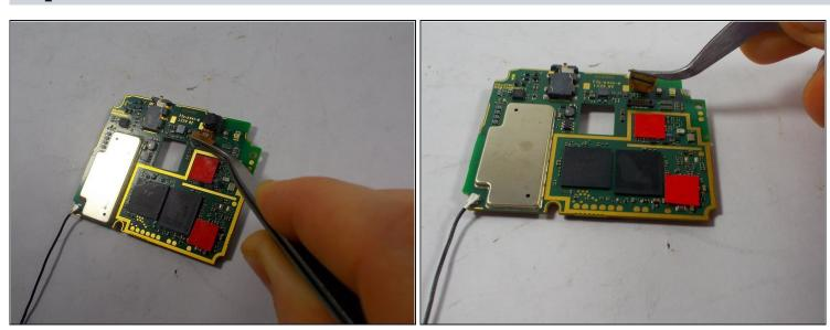
• Use a pair of <u>tweezers</u> to disconnect and remove the front facing camera from the motherboard.
