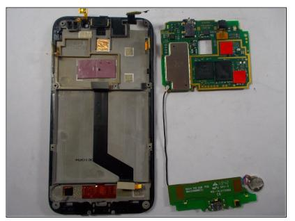
Carefully remove the motherboard from the rest of the phone.
