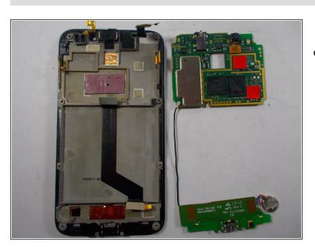
Carefully remove the motherboard from the rest of the phone.
