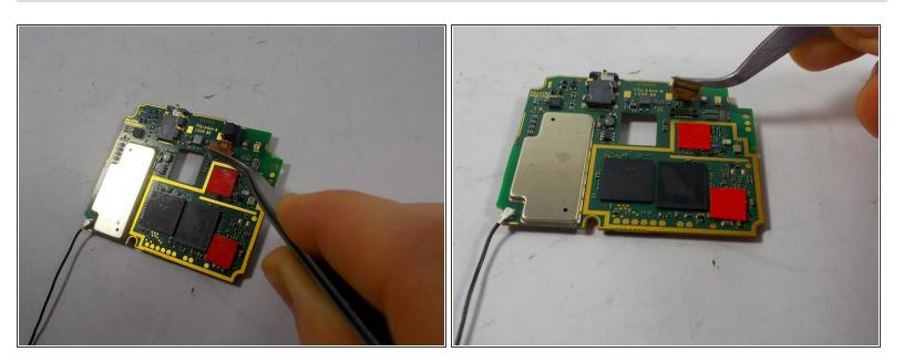
Use a pair of tweezers to disconnect and remove the front facing camera from the motherboard.
