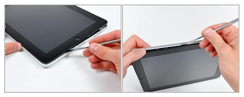
Continue prying the display assembly away from the rear panel along the bottom and left edges of the iPad.
