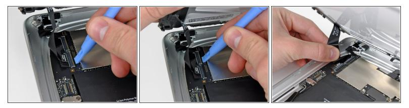
Use the edge of an iPod opening tool to flip up the retaining flaps holding the digitizer ribbon cables in their sockets on the logic board.
