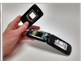
Using plastic opening tool, work around the face plate until it pops off
