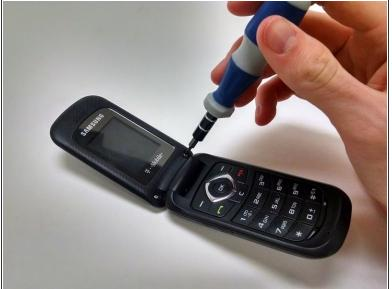
Remove the two Phillips 1.0mm #0 screws
