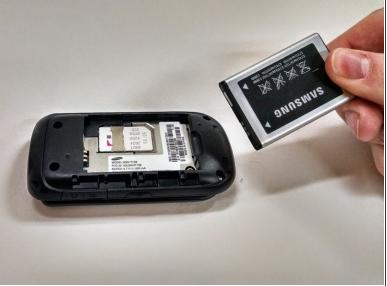
With a plastic opening tool, lift and remove the battery
