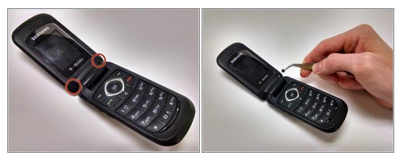
Using the tweezers, remove the two rubber soles that cover the panel screws
