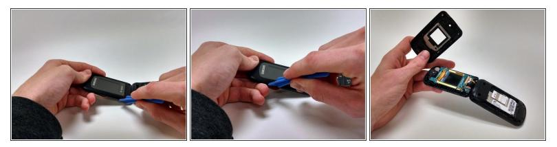
• With the plastic opening tool, work around the face plate until it pops off
