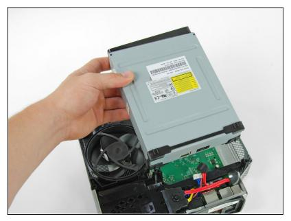
• Lift the optical drive out of the Xbox.
