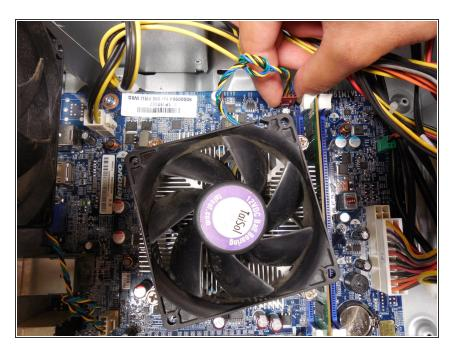
Unplug the fan from the motherboard by gently pulling out the single plug. Then lift the fan up and out of the computer.
