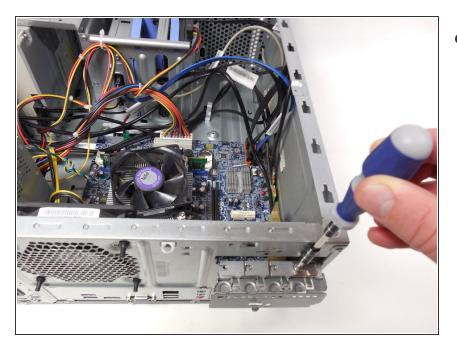
Use the Phillips #2 to remove the 8mm screw that holds the USB 3.0 Expansion Card in place.
